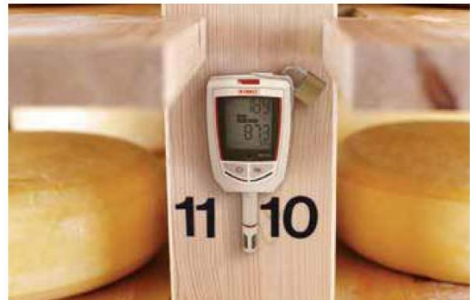
Relative humidity and temperature control in a maturing cellar using a KH 220 mounted onto a plate and secured with a padlock as part of a mapping process
